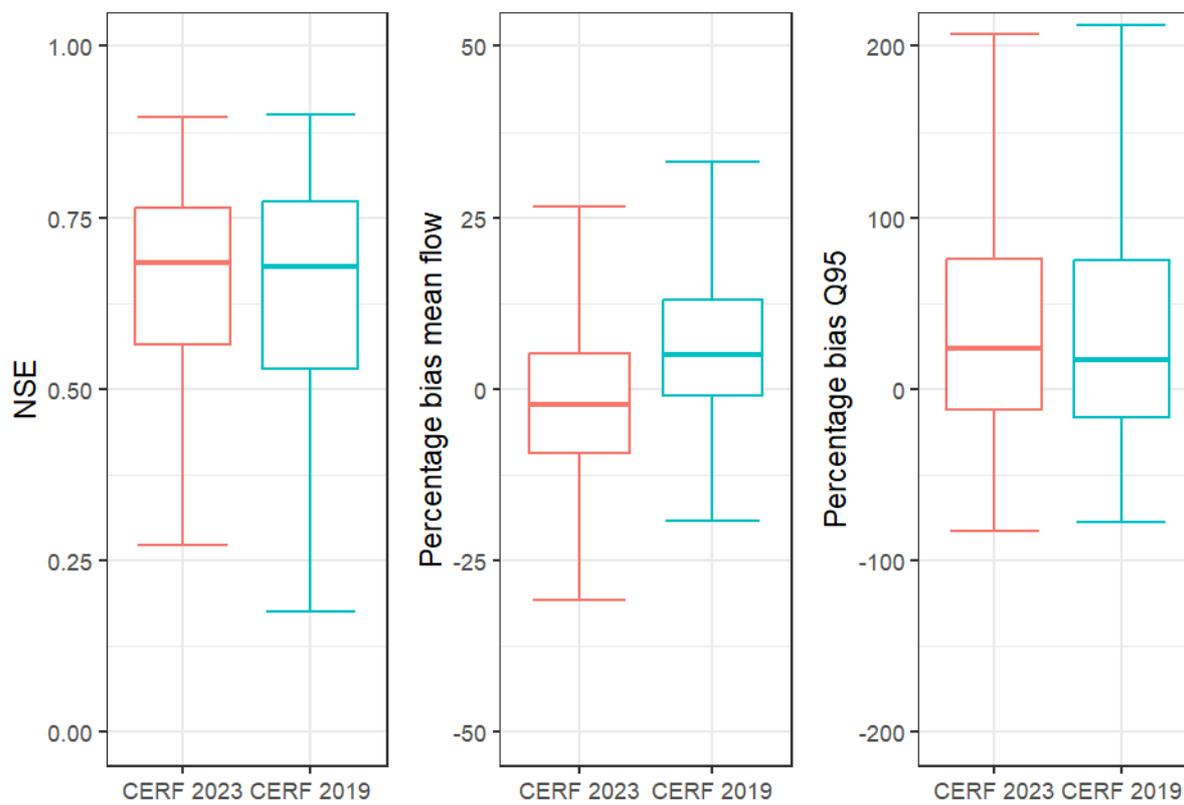
Figure 11. Box plots of the NSE and Percentage Bias at mean flow and Q95 for the coincident gauging stations in the CERF2-HadUK and CERF 2019 datasets. Table 6 illustrates that, in general, all datasets and methods/models perform similarly. There is no one method or dataset that outperforms all others, for all measures of fit. This illustrates the value of using multiple measures of fit, and that the measures of fit should be appropriate for the purpose for which the model is to be used.
