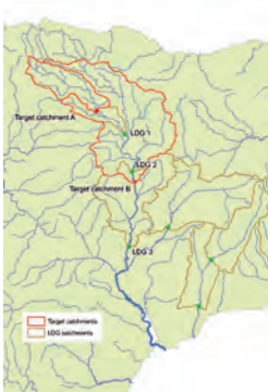
Figure 9.1 LDG 2 is an upstream LDG for target catchment B, LDG 3 is a downstream LDG for target catchment B and LDG 1 is a downstream LDG for target catchment A
